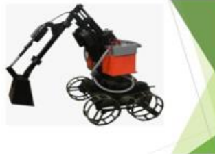
Final year student Harikrishnan Developed The scavenger which automatically clears the block in drainages.
